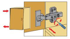
Turn screw clockwise: Door overlay decreases (-). Turn screw anticlockwise: Door overlay increases (+).
