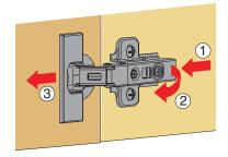
Characteristic for Intermat hinges is the ergonomical snap-on assembly. The hinge is slipped into the front of the mounting plate ①, then a light finger pressure and the hinge arm latches onto the mounting plate ② with an audible click.
