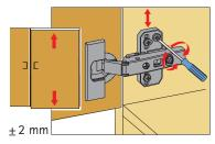
Direct, variable height adjustment with eccentric screw
