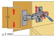
Using height-adjustable mounting plates makes it possible to align the exact door height.
