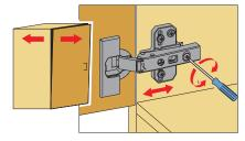
Direct, variable depth adjustment with the eccentric screw
